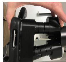
2C Mount connecting oculars to iPad
