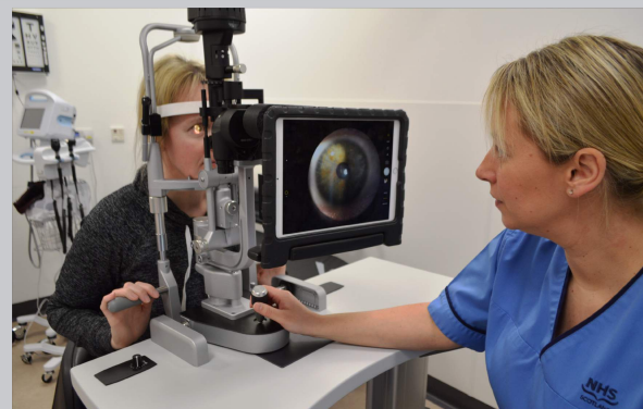
4A. ED slitlamp with bespoke adaptor aligning iPad optics with slitlamp eyepiece. iPad screen serves as digital viewfinder during Skype call across site from hot site (FVRH or MIU) to Falkirk Community Hospital (cold site) on-call ophthalmologist
